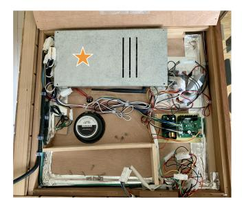
**3.** Loosen the screws on the corners of the power supply unit to access the electronical components of the power supply unit.
