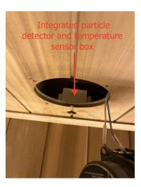
**3)** On the top of this box at the back is the connection for the particle detector. This needs to be removed. Simply pull the connector out of the box by gripping the 3 wires and pulling away from the box.
