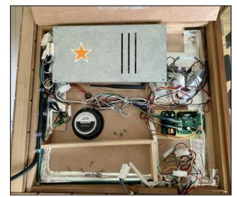
3. Take the new power supply and place it on top of the old power supply. Match the new power supply with the corresponding wires and cords coming out of the old unit. One side will have all male molex connectors and the other will have female molex connectors.
