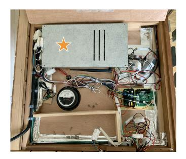
**4)** Locate the connection coming out of the power supply unit or the photoelectric sensor (as shown below), which is the only one with a purple cable.
